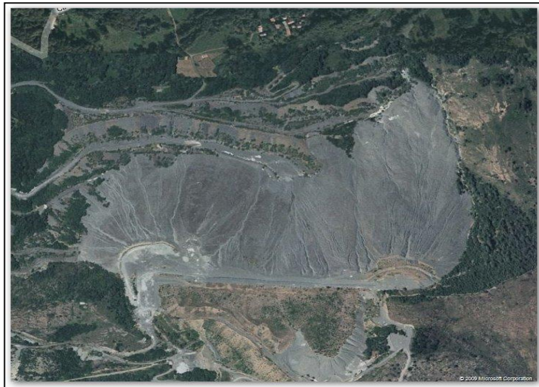
Fig. 1 The Balangero asbestos tailings dump before rehabilitation: 800 m wide, 200–250 m high, slopes between 35 and 45 degrees and an estimated volume of 50-60 Mm 3 .
